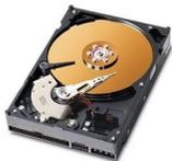
A 3.5-inch SATA hard drive with its top cover removed, showing the internal platters and the actuator arm. |  |
